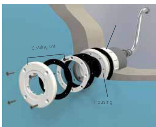
IntelliBrite-E Niche in concrete pool with liner*
