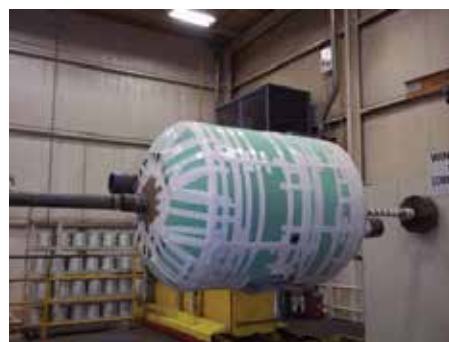
Insulated Vessel at Start of Winding
